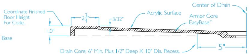
**FEATURES** Dimensional Tolerance  $\pm \frac{1}{8}$ ". Dimensions needed for site preparation should be measured from the unit. Comfort Designs assumes no responsibility for preparatory work.
